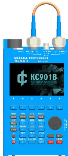
Figure 4-1: Calibration connection when testing with one cable
