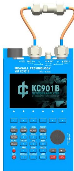
Figure 4-1: Calibration connection when testing with one cable
