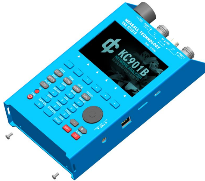
Figure 2-1 Step 1, Remove the bottom screws
