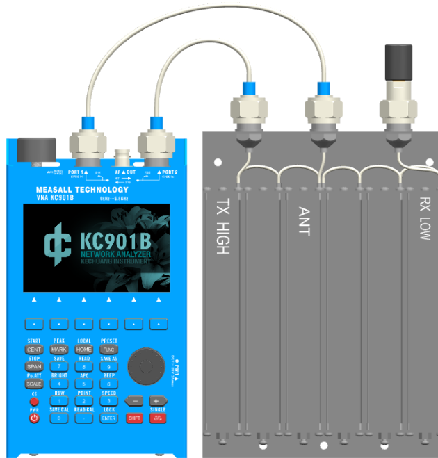
Figure 5-1: Example of test duplexer connection method
